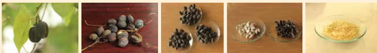
Fig. 1. Experimental materials (a) Fruits in trees, (b) Harvested fruits, (c) separated seeds from fruits, (d) separated husks and kernels, (e) seed powder after grinding
